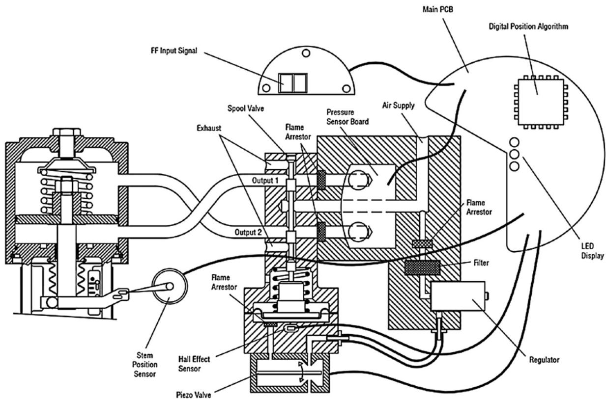
Figure 2: System Positioning Algorithm
