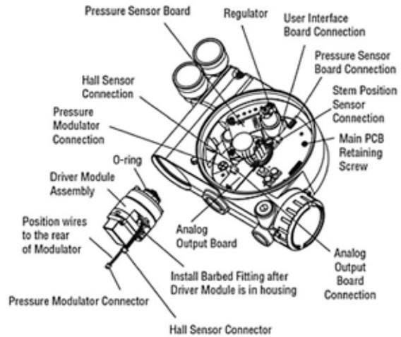
**DANGER:** Spool (extending from the driver module assembly) is easily damaged. Use extreme caution when handling spool and spool valve block. Do not handle the spool by the machined portions of spool. The tolerances between the block and spool are extremely tight. Contamination in the block or on the spool may cause the spool to hang.
